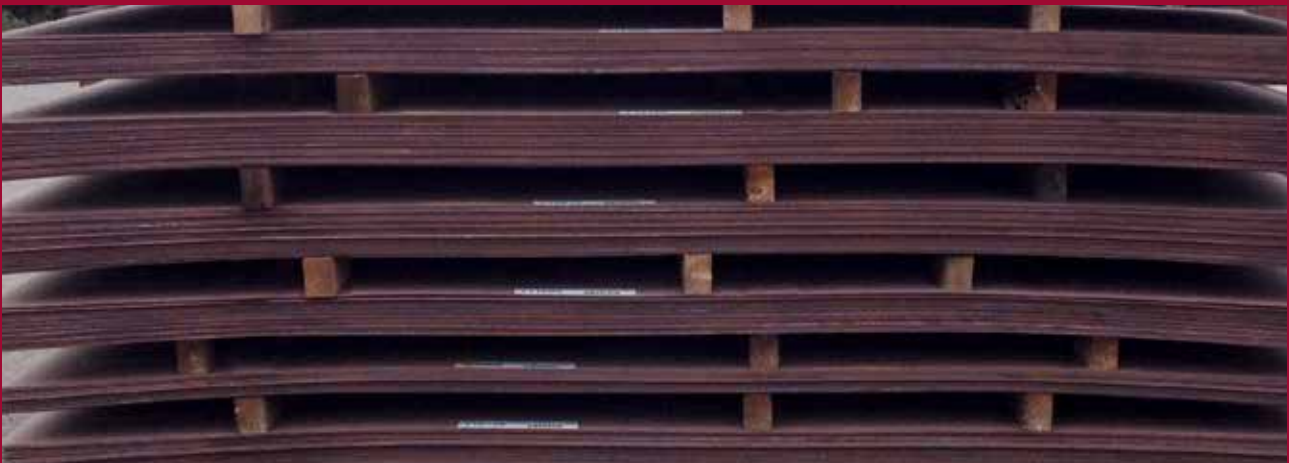
Figure 13b: Improperly stacked plates
