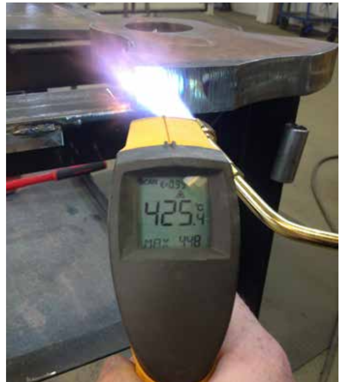
Figure 10: Temperature measurement during postheating.
